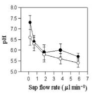
Graph showing the relationship between pH and xylem sap flow rates. As the pH rises, so the flow rates drop.
