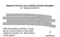
As seen on Page 3, the signal of building movement is far clearer when using levels and above we see why.
